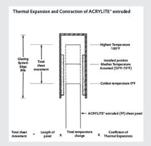
Dark-tinted ACRYLITE® extruded sheets (bronzes and grays) with light transmission less than 60% and facing the south or southwest expand more than colorless sheet due to solar energy absorption. Movement of these panels is about 1.4 times that of colorless or lightly tinted sheet. For 96" (8 feet) of 131-2 Bronze (29% light transmission), it would be:
