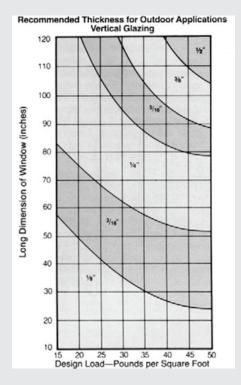
At a design load of 30 psi, glaze a 48"x 36" window with 3/16"-thick sheet. For a 76"x 48" opening, use 1/4"-thick sheet; for a 30"x 12" opening, specify 1/8"-thick sheet. Consult local building code offices tor load requirements in your area. These thicknesses apply to vertically-installed windows only. If your installation is subject to a typical wind load above 30 psi, refer to the following table taken from the drawing above.
