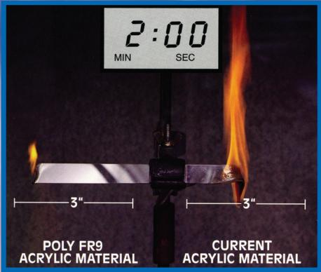
Based on ASTM D635, Polycast POLY FR9 acrylic material burns at about one-fifth the rate of current acrylic materials. Now those who wish to have an environment with low flame spread and reduced smoke generation have a better choice.
