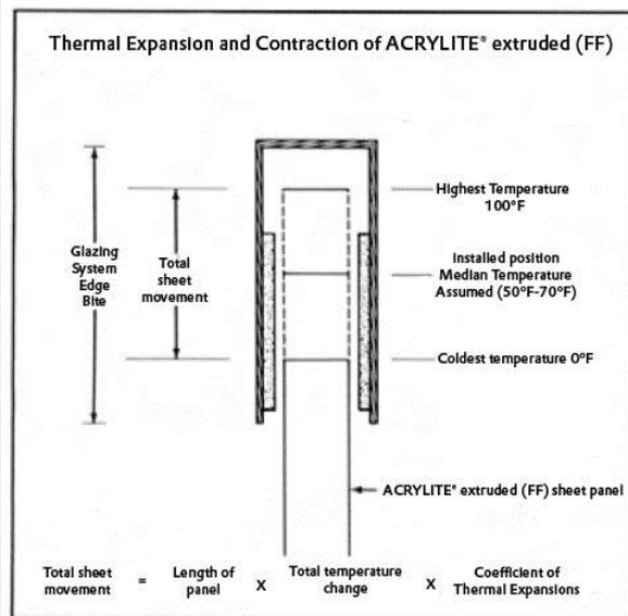
Dark-tinted ACRYLITE® extruded (FF) sheets (bronzes, grays excluding whites and ivories) with light transmission less than 60% and facing the south or southwest expand more than colorless sheet due to solar energy absorption. Movement of these panels is about 1.4 times that of colorless or lightly tinted sheet. For 96" (8 feet) of 131-2 Bronze (29% light transmission), it would be:
