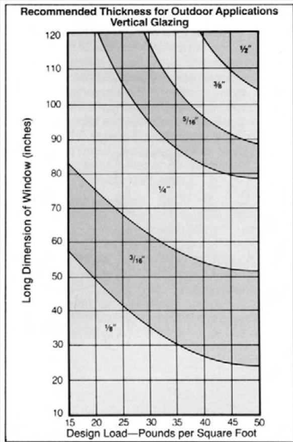
At a design load of 30 psi, glaze a 48"x 36" window with 3/16"-thick sheet. For a 76"x 48" opening, use 1/4"-thick sheet; for a 30"x 12" opening, specify 1/8"-thick sheet. Consult local building code offices for load requirements in your area. These thicknesses apply to vertically-installed windows only. If your installation is subject to a typical wind load above 30 psi, refer to the following table taken from the drawing above.
