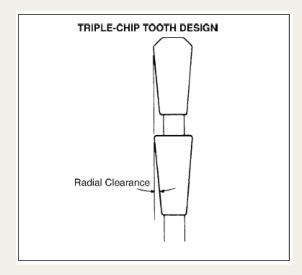
Best results are achieved when the teeth have a clearance angle (top clearance) of 10° to 15°. This minimizes contact between the teeth and the
