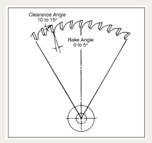
For gang cutting of stacked sheets, a saw blade whose teeth have increased radial clearance is recommended. This clearance will reduce carbide/plastic contact on the sides of the teeth and, therefore, reduce heat generated by friction. When gang cutting, use ACRYLITE® sheet masked with polyethylene masking because it acts as a lubricant.
