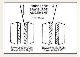
Run-out (or wobble) of the saw arbor and blade collar should be essentially zero. Total run out, including the saw blade, should be less than 0.002". A simple dial indicator to measure the run-out can be purchased from industrial hardware suppliers.
