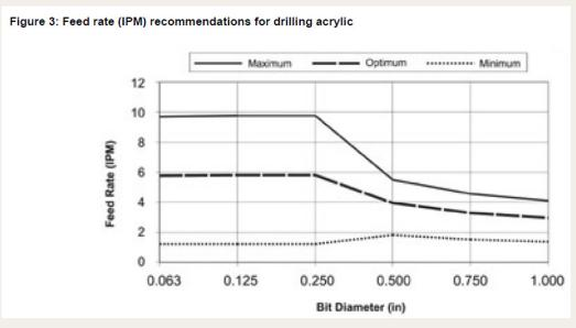
As indicated in the graphs and table on the previous page, lower SFM's are required for larger drill bits. This is to ensure smooth, vibration–free drilling because large bits will tend to grab the material more. As a result, feed rate must generally be slowed down in order to prevent chipping and consequently spindle speed must be reduced to prevent melting.
