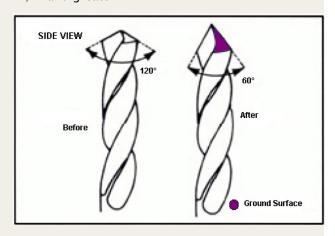
2. The cutting edge must be ground "flat" to a 0-4° rake angle. This cutting edge will scrape the acrylic, not gouge it.
