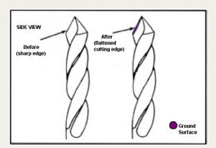
3. The surface behind the cutting edge must be ground away to clearance angles of 12–15°. This back relief reduces metal/plastic contact and heat build-up. This modification is standard on most high quality twist drill bits.
