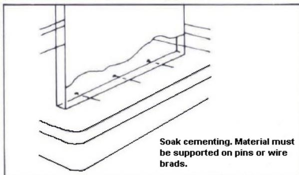
Leave the piece in the solvent 20 seconds for thin sheet and 30 seconds for relatively thick material. The time varies for different solvents and bond strength requirements—experience will help you plan the correct dipping time. Consult Cyro's technical group if you need advice.
