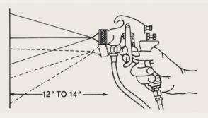
Any efficient atomizing spray gun system, which will uniformly distribute paint, may be used. Consult equipment suppliers regarding the equipment needed for a particular application. Many paint suppliers also publish excellent manuals which provide up-to-date equipment suggestions.
