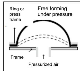
given by the shape and size of the ring affixing it to the frame Vacuum and Pressure Shaping Female Mold.
