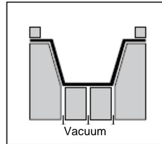
PRESSURE WITH PISTON ASSIST FEMALE MOLD
