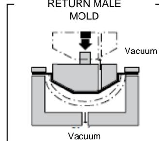
PRESSURE WITH PISTON ASSIST FEMALE MOLD AND VACUUM
