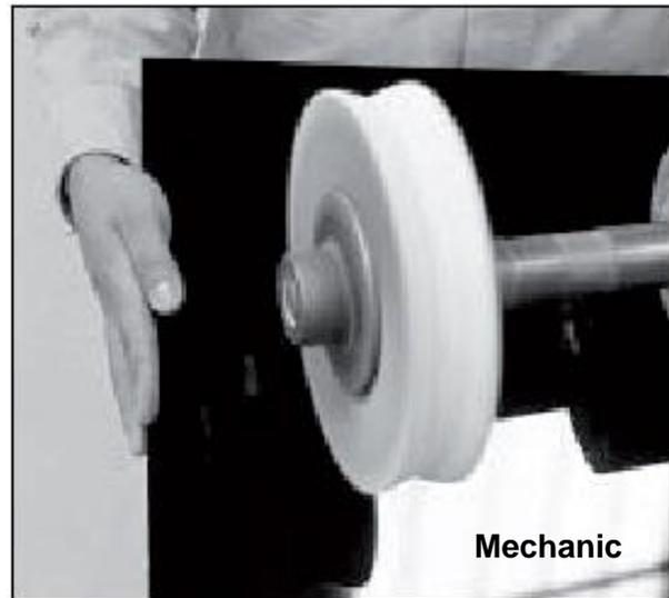
The CHEMCAST acrylic sheet can be polished using a solvent-free commercial polisher, paste wax, or automotive silicone. First apply the polisher to the chamois wheel. Move the piece from one side of the wheel to the other until the surface is evenly smooth and shiny. Be careful, do not apply too much pressure and keep the piece moving in order to keep the sheet from overheating, which could cause burns or disfiguring.
