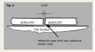
The adhesive is introduced into the one open side of this joint by using a suitable syringe. Avoid bubbles.
