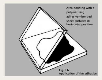
Starting from one edge, the top plate is placed in such a way that the adhesive moves evenly between the plates.
