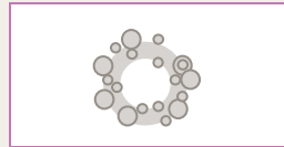
tube – satin texture, optimum light diffusion, extruded
