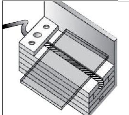
Place the sheet over the supports with the line to be bent directly over the heat line, the material shouldn't touch the walls of the resistance in order to avoid marks.
