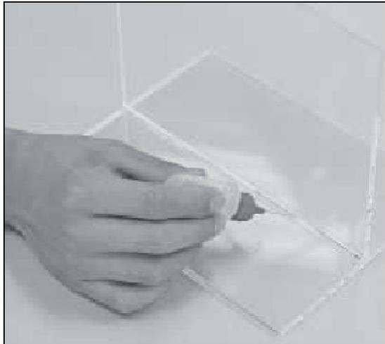
Once the low-viscosity (or edge) adhesive or solvent has been applied, it will flow by capillarity.
