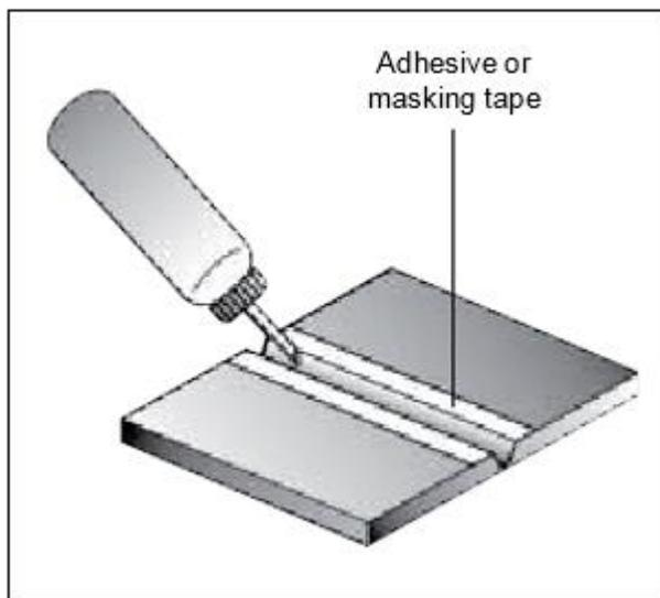
Use adhesive tape to cover the part where the adhesive should not touch
