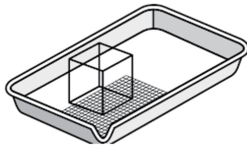
In the submersion method the material should not rest directly on the bottom of the tray.
