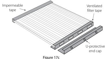
Installation of Impermeable Tape at Top of the Sheet and Installation of Ventilated Tape at the Bottom of the Sheet
