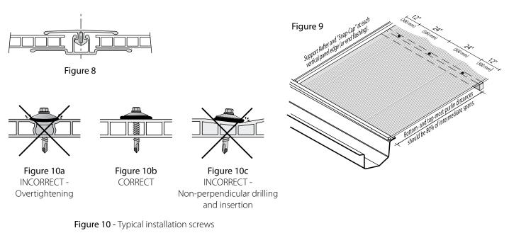
6. Use of self-tapping or self-drilling screws is recommended. In case of wooden structures, suitable wood-screws should be used. All the screws should be corrosion resistant, with at least a heavy-duty hot-dipped galvanized finish. The recommended screw diameter is 6.3mm (1/4 inch). Screw length is selected according to sheet thickness, type of washer, and supporting purlin. In wooden purlins, a minimum of 1 in. insertion of full-size active threads must
