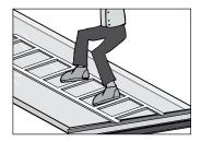
Figure 7 Avoid stepping on the sheets use stepping ladders.
